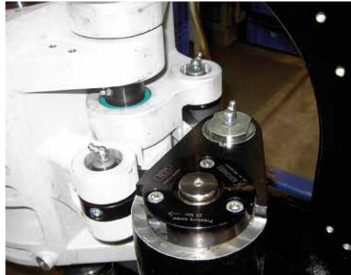
Lever fastened with ETP-EXPRESS to open/close the mould.
