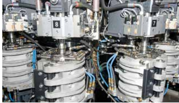
Complete blow mould unit with several moulds/cavities.
